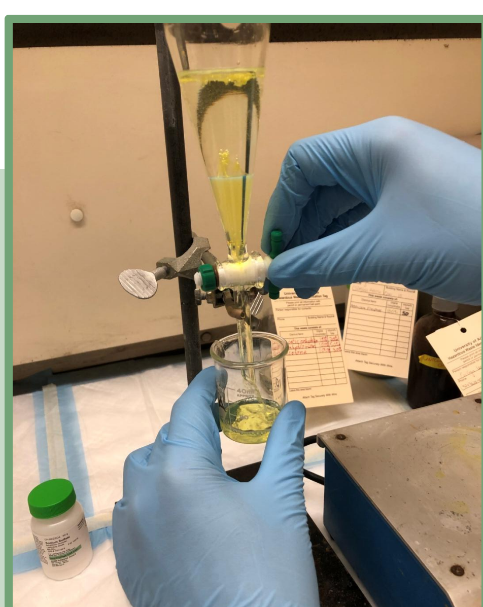
Figure 6- (photo courtesy of exhibitor) Separation of the organic phase which contains the modified photoacid
