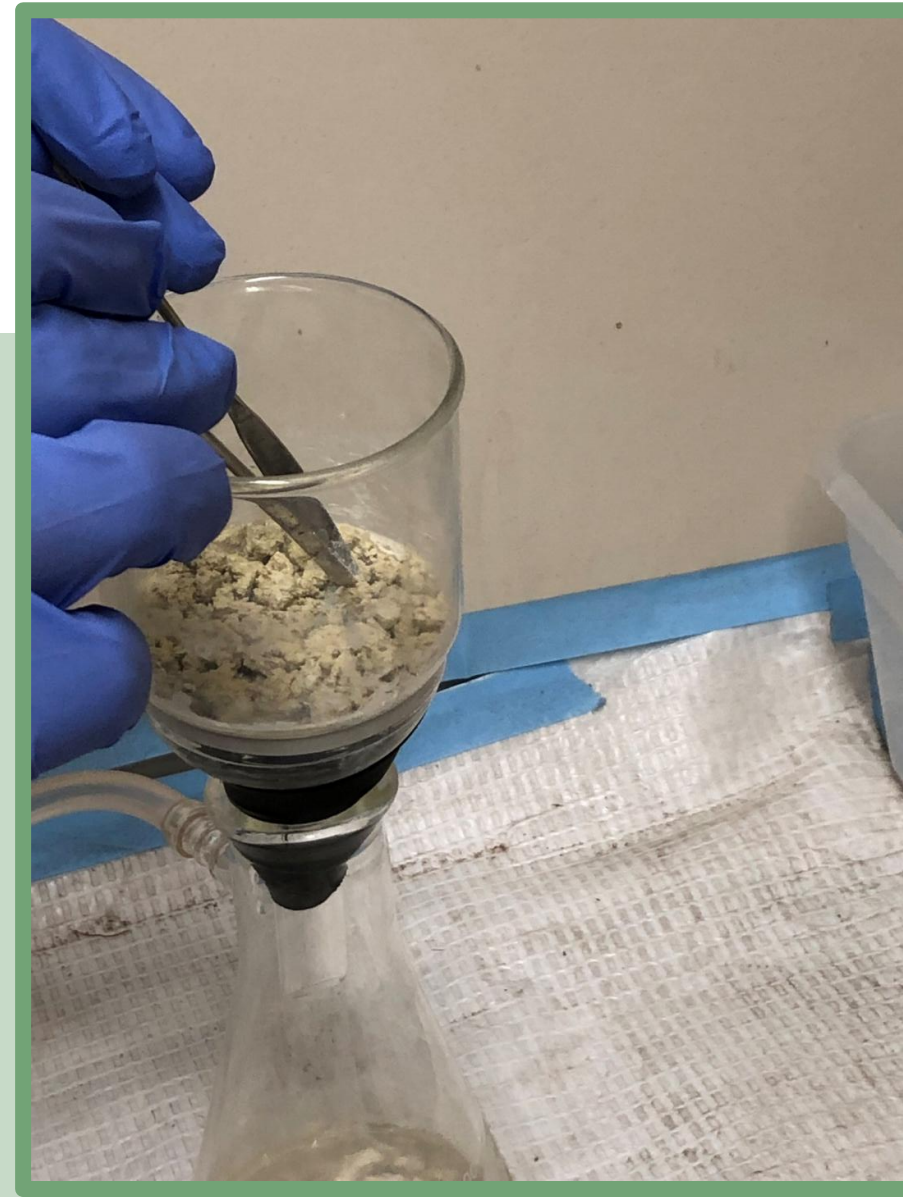
Figure 4- (photo courtesy of exhibitor) Intermediary step in the modification of the photoacid; drying under vacuum
