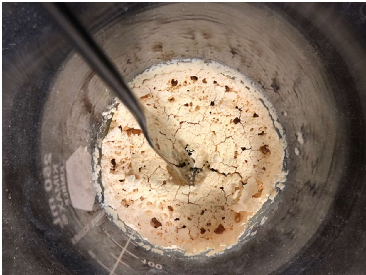
Figure 2– ( Courtesy student ) This picture is of the substance after DCDA is calcined for the first time. It is mostly comprised of graphitic carbon nitride but still contains a significant amount of DCDA. The porous structure is a result of gaseous ammonia escaping and leaving pores during the reaction.
